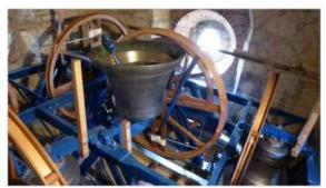
at exactly equal moments in time as it rotated, Big tenor bell ready for laser timing first clockwise then anticlockwise, in relation to its bottom dead-centre rest position.
